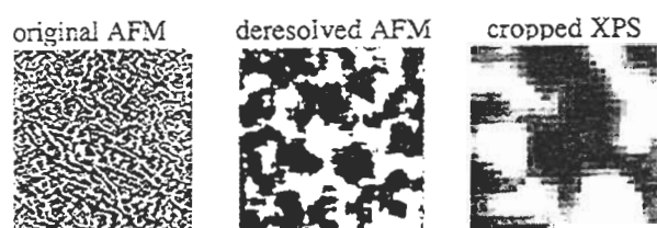
Figure 9. Comparison of original, deresolved AFM and cropped XPS imaged from 50%/50% PVC/PMMA blend
